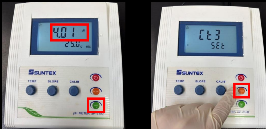
Figure 16. Calibration schematic diagram of the new model pH meter.
