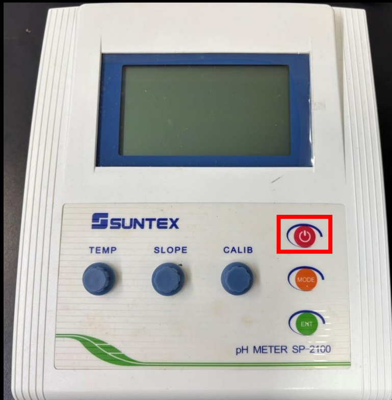
Figure 12. Startup procedures for the new model pH meter.
