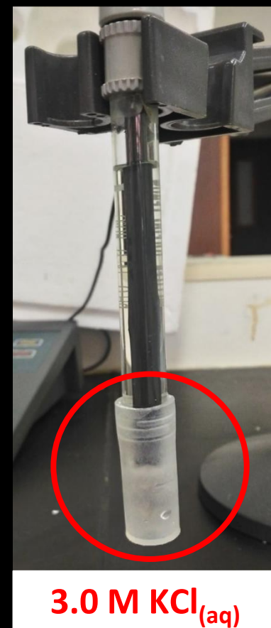
Figure 20. Schematic diagram of the KCl electrode cap.
