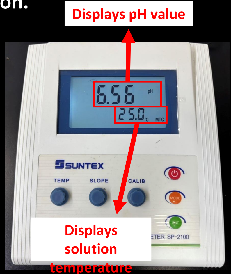
Figure 12. Startup procedures for the new model pH meter.
