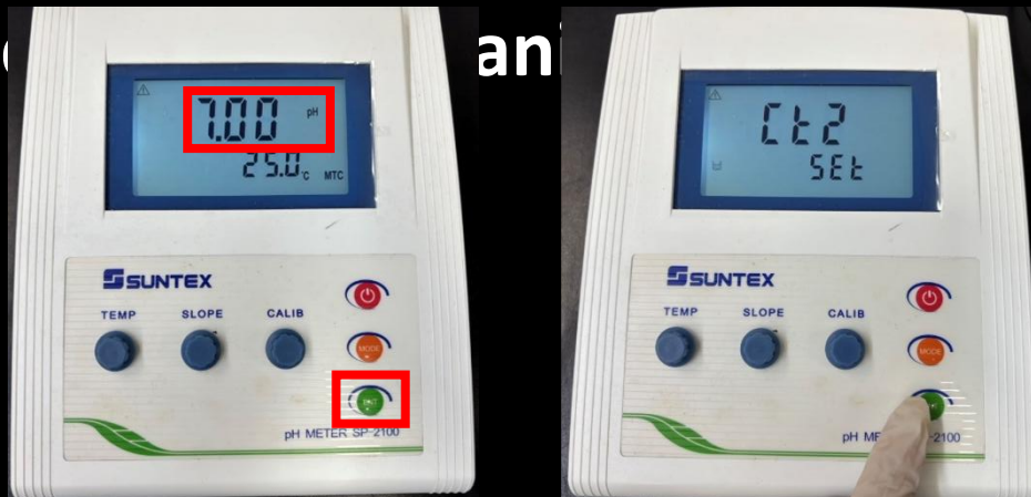
Figure 15. Calibration schematic diagram of the new model pH meter.
