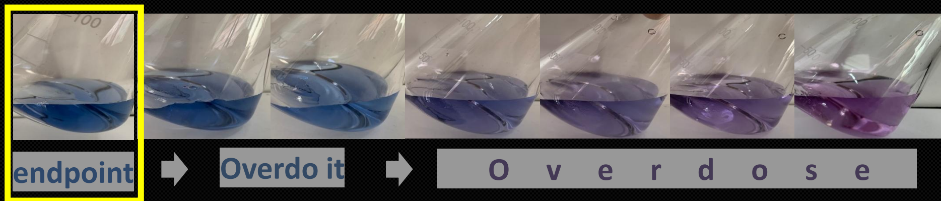
Figure 7. Titration endpoint color and titration excess color change.
