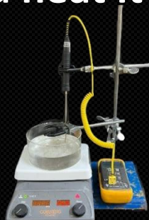
Figure 2. Experimental setup for conventional heating.
