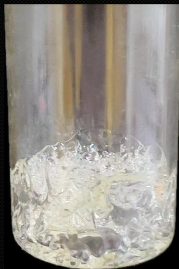
Figure 1. PVP solid prepared by microwave heating.
