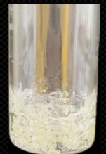
Figure 3. Poly(vinylpyrrolidone) (PVP) solid prepared by conventional heating.
