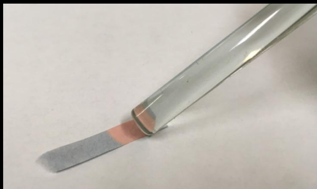
Figure 5.4 – The blue litmus paper turned red, confirming that the solution is acidic.
